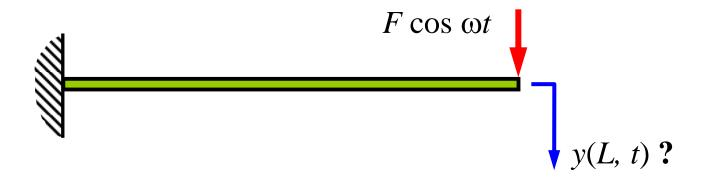
**Objective:** Use a single-degree-of-freedom model to estimate the steady-state response at the free end of a uniform cantilever beam due to a sinusoidal force with a frequency near the lowest natural frequency of the beam
