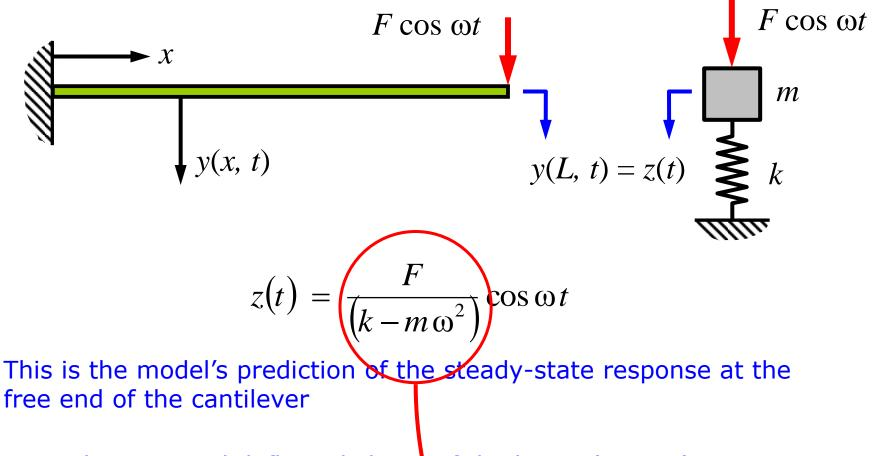
From the assumed deflected shape of the beam (eqn. A), we can find the vibration amplitude at **any point** along its length
