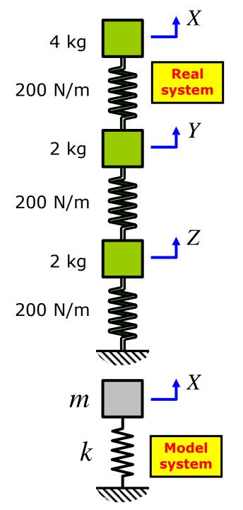
Equating max. **kinetic** energies in the real and model systems
